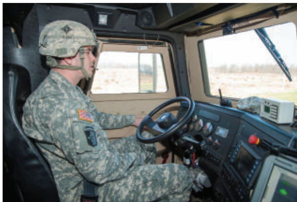
U.S. Army vehicle electronics researchers use the line-haul tractor to explore driver-optional capabilities, from driver-assist features to autonomous leader-follower or waypoint-navigated driving.
