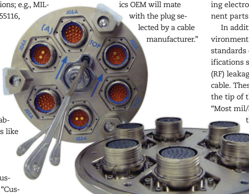
Eaton's umbilical connector facilitates first-stage separation in launch-vehicle applications.
